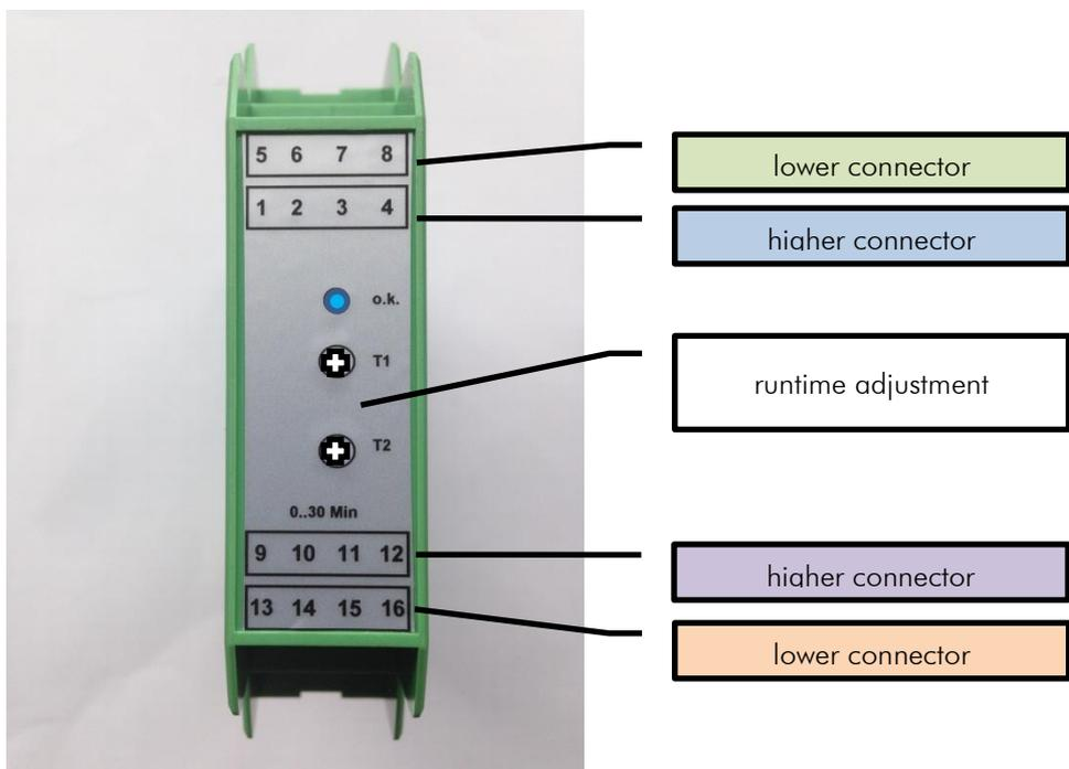
Notice: „higher“ and „lower“ refer to the distance from the mounting plate up to the connectors
